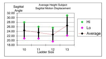
In order to try to further interpret the sagittal bending data, we calculated range of motion between the peak fluctuations, plotting the average range of motions for each ladder in the figures below. Table 19 below shows lower relative fluctuations for the 11 and 12 inch ladders at about 2.5 degrees, with the 13 inch ladder producing the largest fluctuation with a value of about 4.7 degrees.
