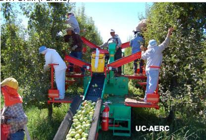
California pear trees are among the tallest and largest of hand-harvested tree crops, often requiring 14-16' ladders. The intended advantage of the powered platform is to completely eliminate ladder use and risk altogether. For the pear harvest platform trial a Spanish built Argiles self-powered platform was provided by BlueLine Manufacturing of Yakima, WA. The machine required extensive modification by UC AERC staff to meet the demands of pear harvest.
